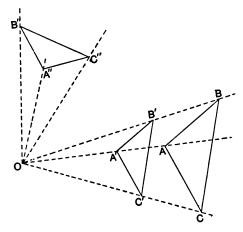
Let A'B'C' be any triangle having its sides parallel to the corresponding sides of the triangle ABC; and let O be the centre of perspective. Since the corresponding sides are parallel, it follows at once that
